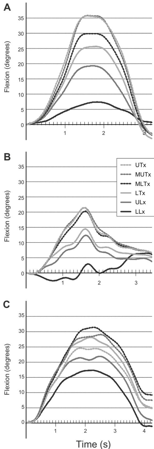
**Fig. 4.** Cumulative flexion motion patterns at each trunk level within the multi-segmental model, for three subjects, for a single trial toward an anteriorly placed target at distance 3. Cumulate motion is presented to each visual comparison, with the motion illustrated for each level representing the summed motion for that level with each more caudal level (e.g. the motion pattern illustrated for LTx is the summed motion for LTx, ULx and LLx).
