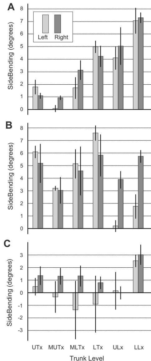
**Fig. 5.** Side-bending motion, at the point of peak trunk motion, at each trunk level within the multi-segmental model, for three subjects, during movement toward the targets placed in the frontal plane at distance 2. Bars represent the mean trunk motion over three trials. Error bars represent a range of plus or minus one standard deviation.
